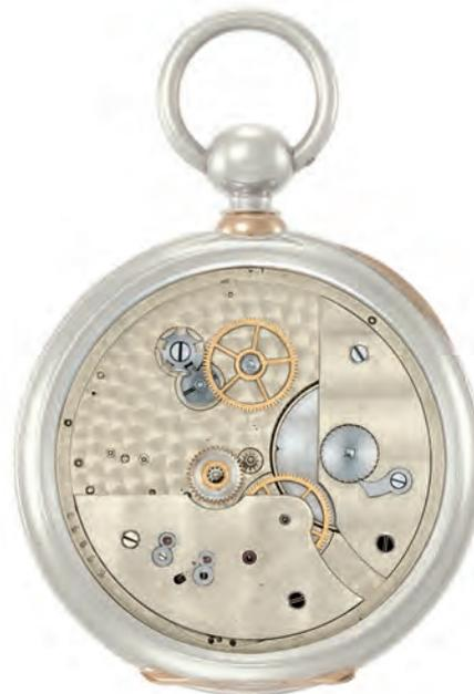
**Pocket Chronometer with Spring Detent Escapement,
