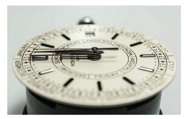
Unusually, there are 5 central hands on the dial of the REF. 5212A. They indicate hours, minutes, seconds, the week number and day of the week. There is also a date in an aperture at three o'clock. Correction of the day and number of the week is via pushers at eight and ten o'clock respectively, while the date is adjusted via the crown
