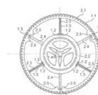
1/10 driving wheel with anti-backlash feature (European patent EP3042250B1)
